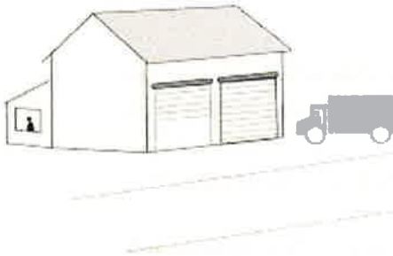
Fig. 5a. NO. Locating utility areas directly toward a right-of-way can create an unattractive edge to a scenic highway, and does not provide an understandable entrance for customers/clients.
