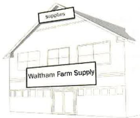
Fig. 6a. NO. Signage out of scale to building and covering unique architectural details.
